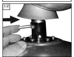
Insert downrod into motor yoke. Next, insert clevis pin through yoke and downrod.
